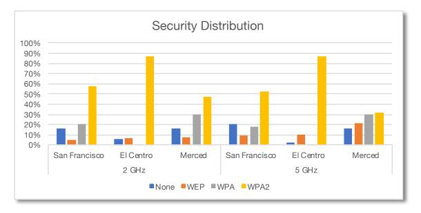
What we can evaluate is the quality of the encryption regime given a strong encryption key<sup>9</sup>. Sadly, many users have chosen to use no encryption or legacy encryption standards such as WEP and WPA that are weak with known vulnerabilities.
