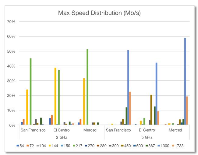
Looking at the type of modulation, we can make an estimate of the generation of WiFi included in a gateway. Very early (pre-standard, so-called "draft n" access points (likely deployed circa 2007) 802.11n gateways used single band 2 GHz operation (no 5 GHz service) with very limited use of MIMO (no more than 2x2 in 20 MHz channels). These were often deployed with carrier deployed DSL gateways where the limited WiFi throughput matched the limited throughput of the carrier connection.
