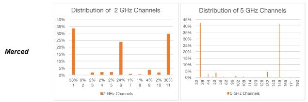
5 GHz channel usage is interesting. Older 5 GHz technology, like 802.11n, only support 20 and 40 MHz wide channels. Modern 802.11ac supports 20, 40, 80 and 160 MHz channels. In all three cities, 80 MHz channels are the majority, but El Centro shows a strong minority use of 3x3 MIMO 802.11n in 40 MHz channels (and in 20 MHz channels at 2 GHz).
