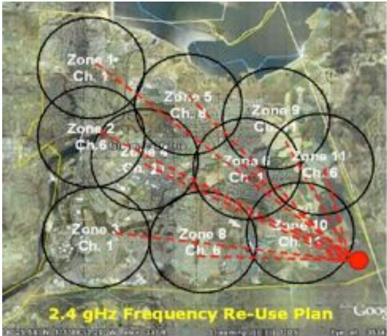
Figure D5. 2.4 GHz WiFi Frequency Re-Use Plan. WiFi Zone Diameter = 1.5 miles range assumes point-to-point directional antennas from Hot Spot Access Point to end-user.
